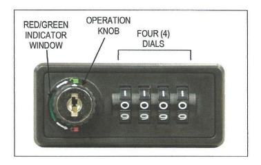
The lock has a four (4) digit combination setting. When the lock is locked (closed), a red indicator appears in a window next to the operation knob. When the lock is unlocked (open), a green indicator appears in the window.
