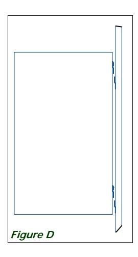
**Step 3:** Install the second Bracket to the wall. Positioning should be determined by the distance that was measured in **Step 2**.
